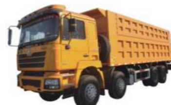
Brand:SHACMAN 8*4 LHD/RHD Engine: 340HP, 350HP, 380HP Loading Capacity:35T - 45T
