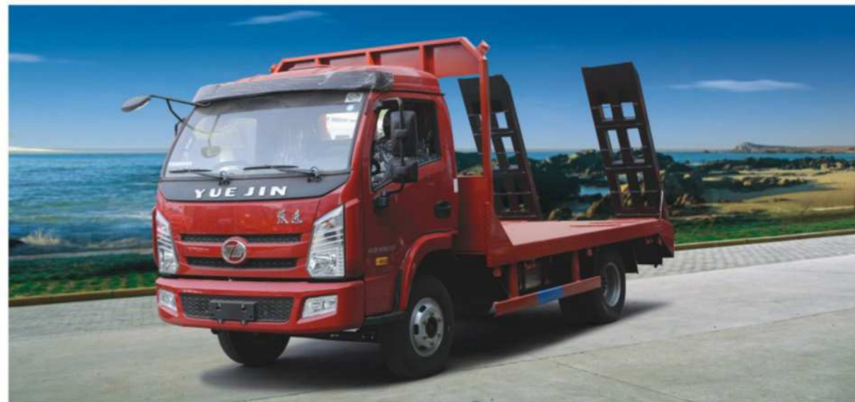
Yuejin Self loading truck (90HP-130HP,6-8 tons,flatbed length:4.7m )
