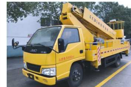
16 Meters Telescopic Booms Aerial Platform Truck
