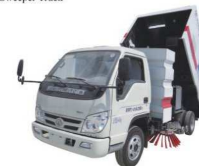
Foton 1.5 water tank & 3-4 m3 dust tank
