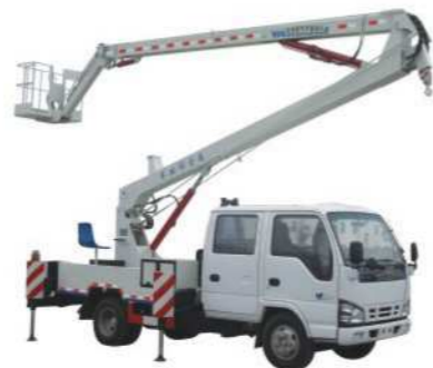
Brand :ISUZU 4*2 LHD Engine : 98HP Working Height :10-16m
