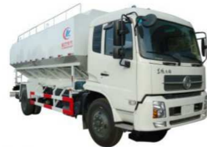
Brand: Dongfeng 4x2 LHD RHD Engine: 160HP, 170HP, 190HP, 210HP Volume: 20m 3
