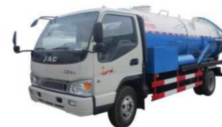
JAC sewer dredging vehicle, 3m3 water tank and 4.5m3 sewage tank
