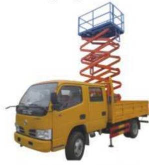
Brand : Dongfeng 4*2 LHD or RHD Engine : 95HP Working Height :6-12m
