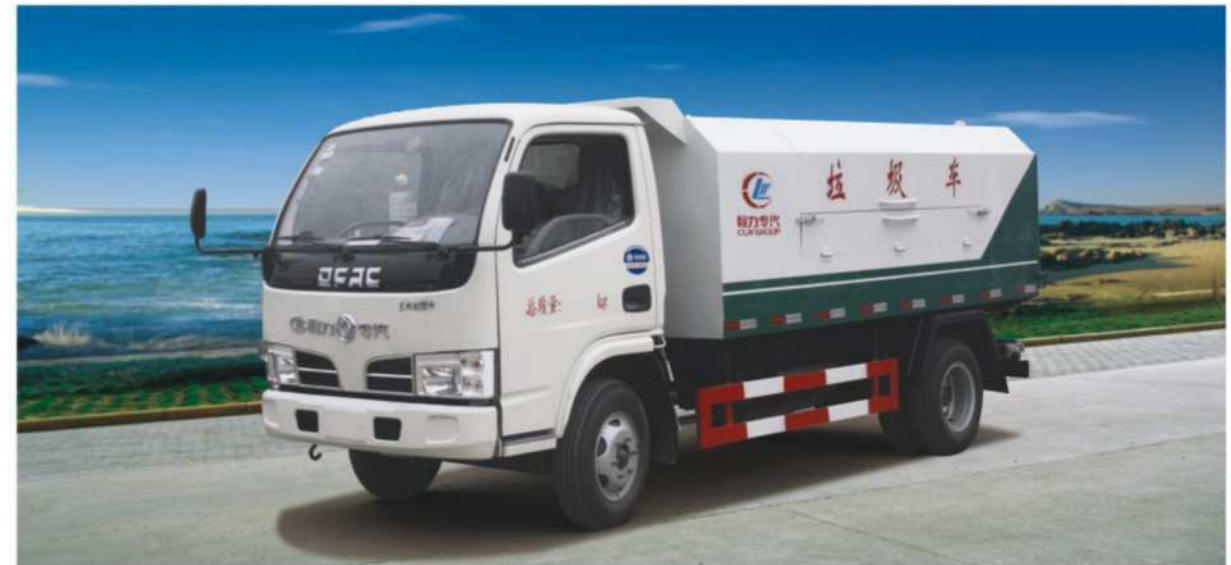
DONGFENG Sealed dump garbage truck, CHAOCHAI engine 95hp,4-5m3
