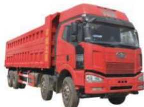
Brand:FAW 8*4 LHD/RHD Engine: 340HP, 350HP, 380HP Loading Capacity:35T - 45T
