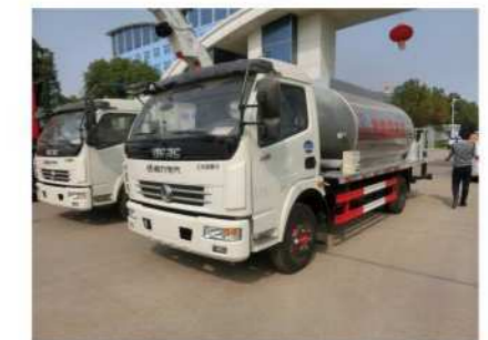
DFM/JAC/JMC/ISUZU 4m 3 -6m 3 Asphalt distribution truck
