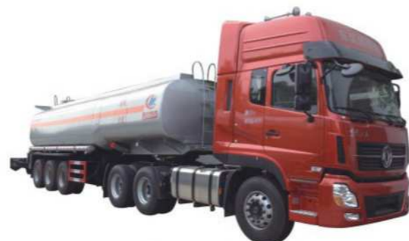
3 axles 48CBM fuel tank semi trailer
