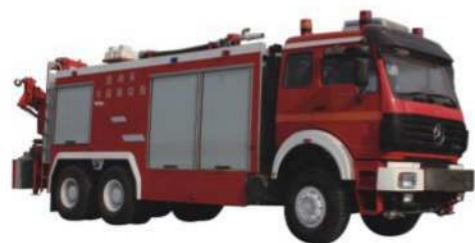
North Benz, Engine 340hp, Volume: 10-12m 3
