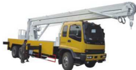
Brand :ISUZU 6*4 LHD Engine : 280HP Working Height :20-28m
