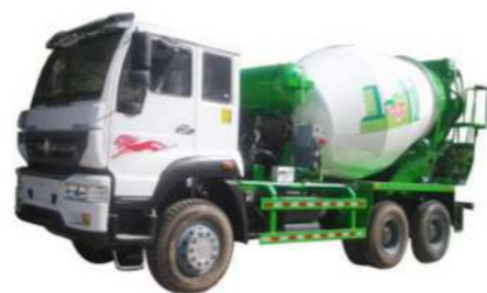
Brand: SINO styre 8x4 LHD or RHD Engine:340HP, 380HP Volume: 8m3 to 16m3
