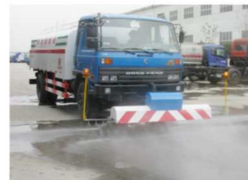
Dongfeng road flushing truck, 8m3 tank, 170hp
