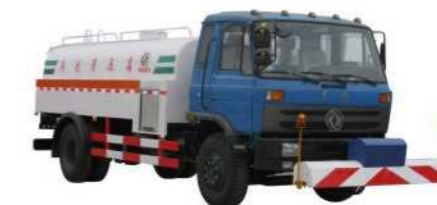
Dongfeng road flushing truck, 8m3 tank, 170hp
