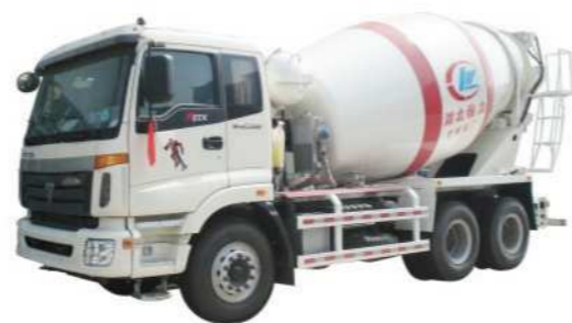
Brand: Foton 6x4 LHD Engine:266HP,290HP,336HP,380HP Volume: 6cubic meter to 12cubic meter
