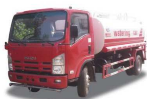
ISUZU water tank truck,engine:ISUZU 190hps, volume:6-8CBM
