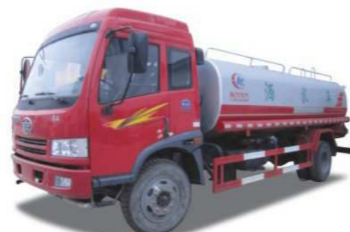
FAW water tank truck, engine:Xichai 180hps, volume:8-10CBM
