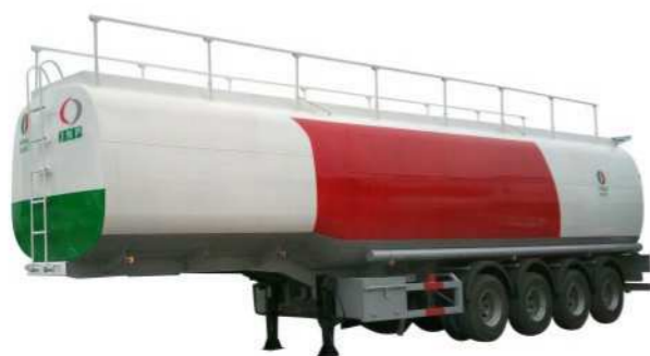
3 axles 60CBM carbon steel fuel tanker semi trailer
