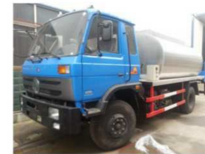
DFM(Dongfeng) 9m 3 Asphalt distribution truck
