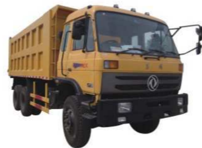
Brand:DONGFENG 6*4 LHD/RHD Engine: 210HP,260HP Loading Capacity:15T - 30T
