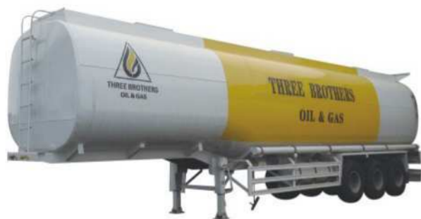
3 axles 56CBM carbon steel fuel tanker semi trailer
