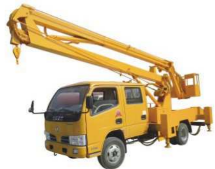
Brand : Dongfeng 4*2 LHD or RHD Engine: 80HP, 95HP, 102HP Working Height :10-16m
