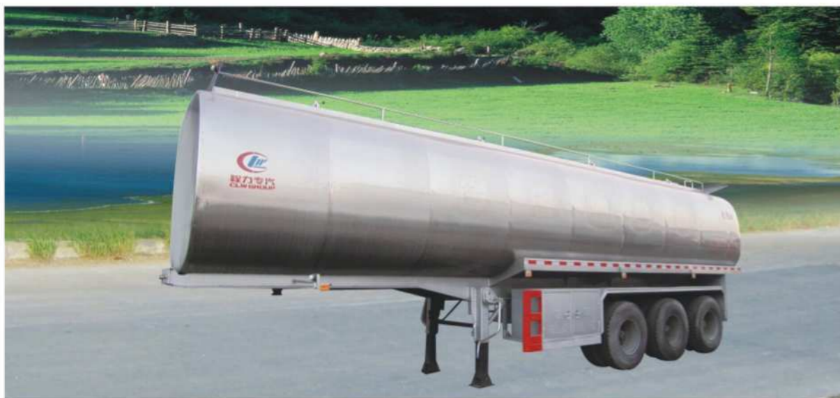
3 axles 50CBM stainless steel fuel tanker semi trailer
