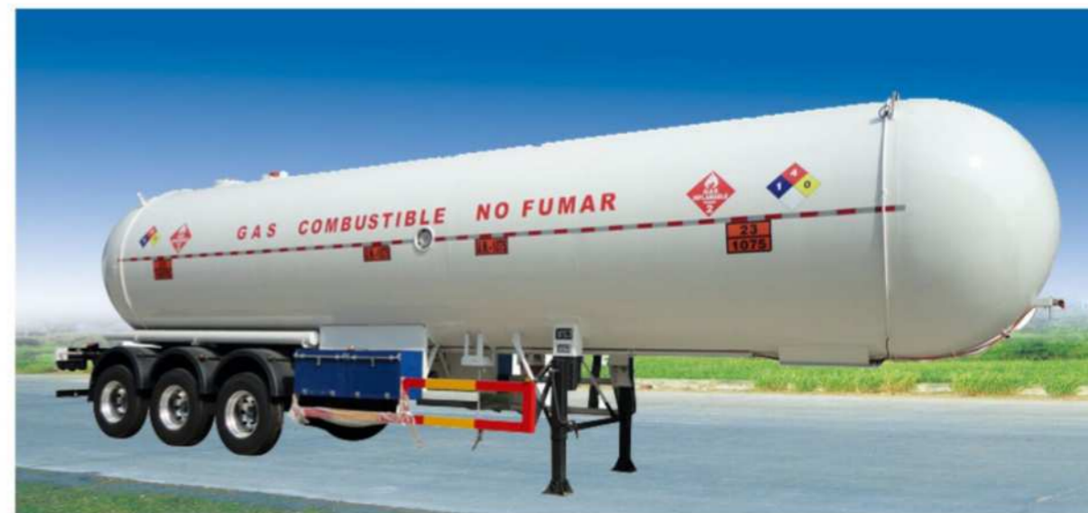
Material: Q420R/Q370R/Q345R/ASME SA516 Pressure: 1.61Mpa Tank Volume: 40.5CBM-59.52CBM Medium: Propane/Liquefied Petroleum Gas
