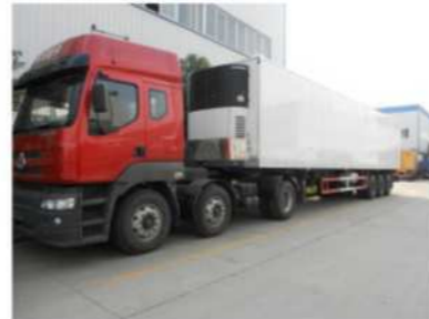
3 axles 40 feet Refrigerator trailer with Carrier units
