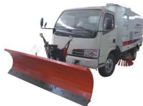
DONGFENG 5m3 Road sweeper truck with Snow shovel
