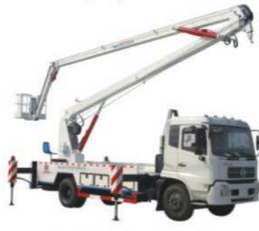
Brand :Dongfeng 4*2 LHD Engine : 160HP ,180HP ,185HP Working Height :18-24m
