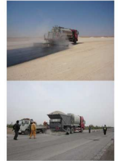
Howo 6*4 asphalt distribution truck, 10m 3 -12m 3 , Intelligent automatic control/ half automatic control
