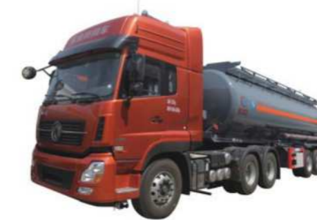
3axles Chemical tank trailer, 30cbm sulphuric acid tank
