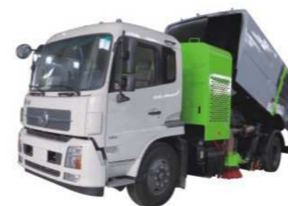
Dongfeng cleaning sweeper truck, 7m3 dust tank & 3.5 water tank
